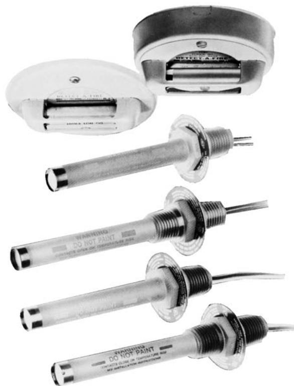
The secret of the unit's sensitivity is in the design (Figure 1). The outer shell is made of a rapidly expanding alloy which closely follows changes in surrounding air temperature. The inner struts are made of a lower expanding alloy. Designed to resist thermal energy absorption and sealed inside the shell, the struts follow temperature changes more slowly.
